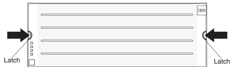
Figure 80. Removing the bezel
